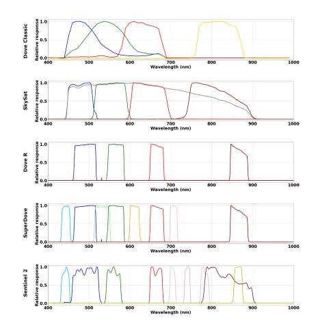
Figure 2: Relative spectral response curves of Planet's payloads
