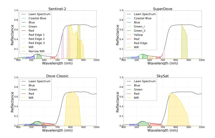
Figure 3: A lawn grass spectrum from a spectral library for (A.) Sentinel 2A (B.) SuperDove (C.) Dove Classic and (D.) SkySat
