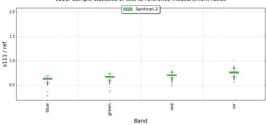
s111: Sample statistics of test to reference measurement ratios
