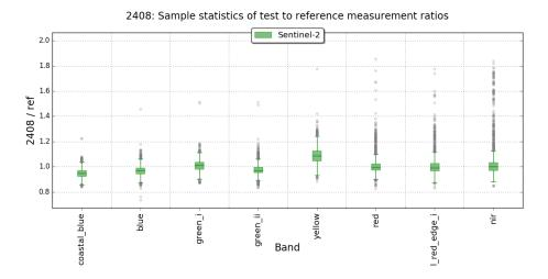
The calibration gains derived from these comparisons to Sentinel-2 were used to generate corrections to the calibrations that became effective at the end of Q3 of 2021. Figure 19 shows the distribution of calibration gain updates for all the SuperDove satellites within this update.
