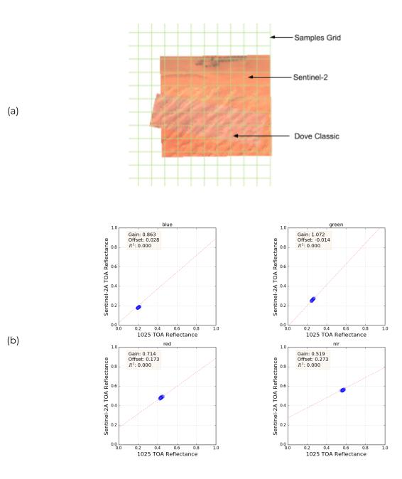
The joint modes (or mean values in the case of SkySat crossovers) of all the individual scene pairs are then collected and a RANSAC fit is used to calculate the gain and offset for each band. For SkySats, the RANSAC fit is forced through the origin. The Dove Classic example has many more data points in the final regression than the SkySat example due to the fact that Doves constantly monitor whereas SkySats are tasked satellites.
