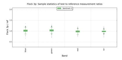
These crossover results were combined with lunar trending data for each satellite to derive the per-satellite corrections. Not all Flock 3p satellites had sufficient quality data to derive a lunar adjustment factor. For those that didn't, the baseline flock wide correction was used. Figure 15 shows the distribution of gain correction factors that were applied to Flock 3p satellites. These new calibrations became effective at the end of Q3 of 2021.
